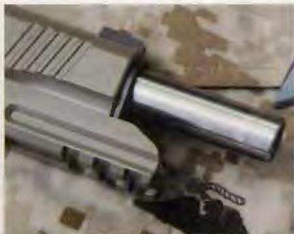
As specified by the USMC in its original Kimber, the Warrior comes without a full-length guide rod for ease of maintenance in harsh environments.
